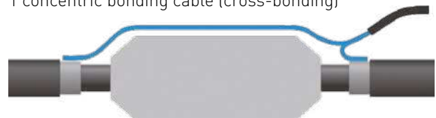
MSA XK Screen interrupted with 1 concentric bonding cable (cross-bonding)
